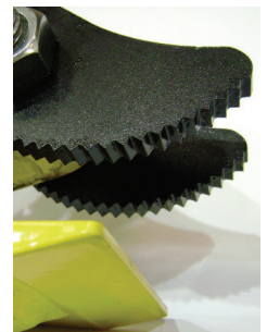
***CH with serrated jaw which can only be used for single plates, NOT bundles.
